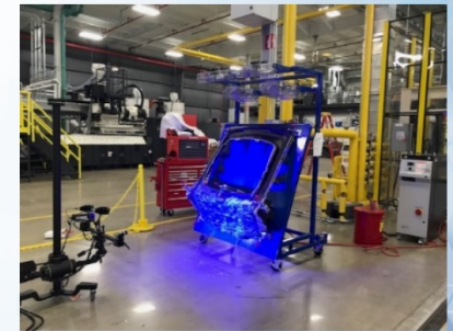
Digital Image Correlation (DIC) for fiber orientation
