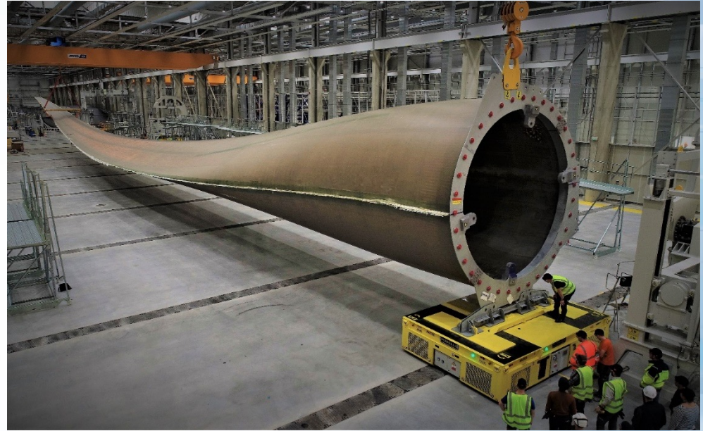
107m blade for 12MW offshore turbine
