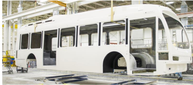
Proterra Bus Body Structure Assembly
