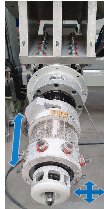
3D-Aggregate with surface copying function in 3 axis
